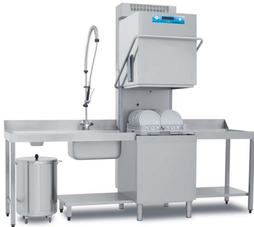
River 83 hood dishwashers can be equipped with the NRG heat recovery/steam condensation system. At the end of rinsing, the steam in the wash chamber is extracted and routed to a heat exchanger where it condenses and gives up its heat to the intake water.
