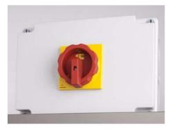
Isolating switch on the machine
