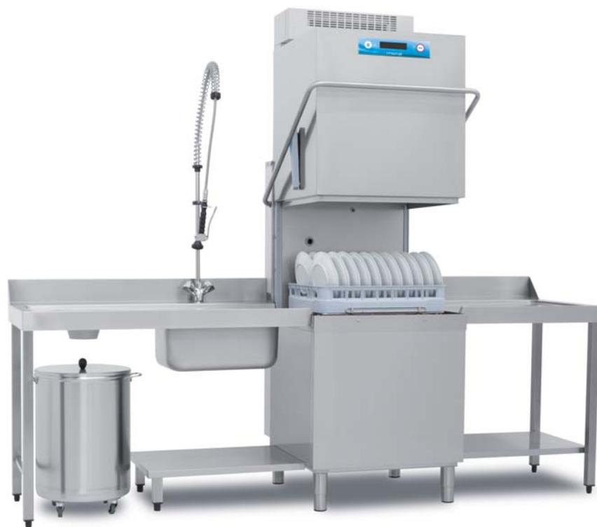
Both Mistral 94LX hood dishwashers can be equipped with the NRG heat recovery/steam condensation system. At the end of rinsing, the steam in the wash chamber is extracted and routed to a heat exchanger where it condenses and gives up its heat to the intake water.
